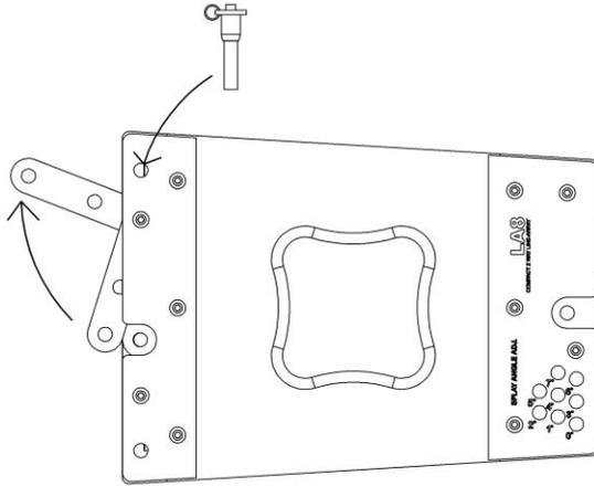
1. Pull the front joints out and insert a lockpin on the alignment hole. This lockpin will hold the joint in place and prevent the system from articulating while in the air. **Check if the pin is locked on.**
