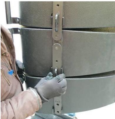
One per side: grab the side handle in order to hold the loudspeaker once the side bars have been removed.
