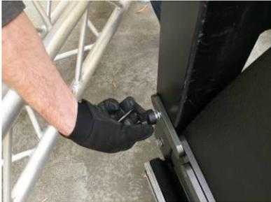
Screw the handle and accompany the bar in its position in order to lock it to the frame and to the first loudspeaker.
