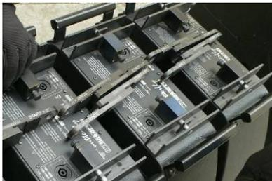
Prepare the pairs of back connection bars previously set for each loudspeaker.
