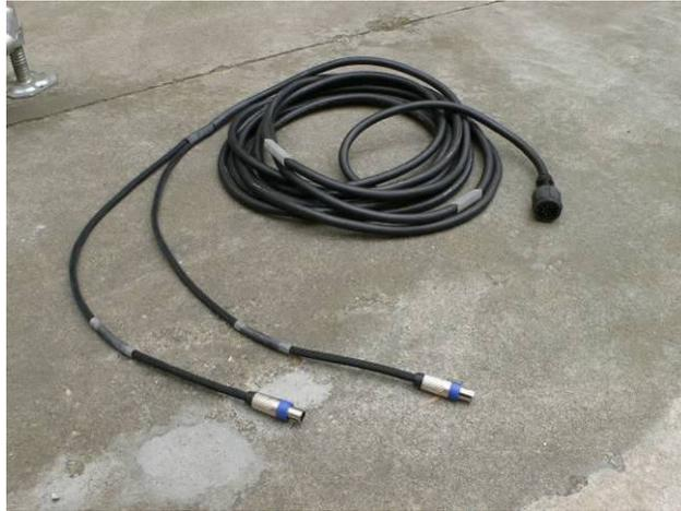
The recommended speaker cables have one end (rack side) with a male 8-pole connector and two Speakon NL4 (loudspeaker side). Each NL4 drives two butterfly in parallel or three Mantas using 4-wire cable with one NL4 connector on each side. Please respect the suggested amplifier configuration
