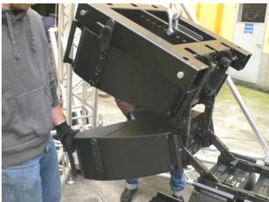
One per side: grab the second loudspeaker by the front handles and prepare it for the following connection to the front.
