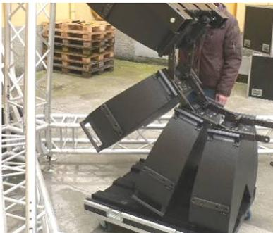
Keep on lifting in order to raise the second loudspeaker as well.
