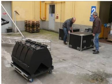
Remove the flight-case cover and prepare the pack of loudspeakers into position to be rigged. Prepare also all the speaker cables (not shown here) and remove the side bars from their rest position.
