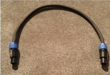
0.7 m bridge cable for loudspeakers.
