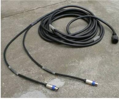
25 m long cable to connect the amplifier rack with the loudspeakers (SP2 LK18-25). Each complete rack will require three cables like this one.
