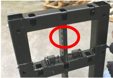
In case of extreme array up-tilting, the extension can also be connected to the front of the main frame. Remove the central bar by removing the two screws (image on the left). If the application requires the use with a single motor the central bar has to be substituted by the specific shorter one (A BAR-254).
