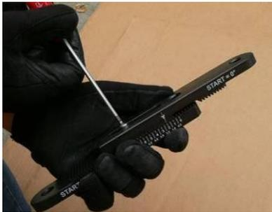
**Don't use excessive torque to tighten the screw, use just the force needed in order to have no mechanical lash (although a very small lash is admitted).** This will facilitate the installation.
