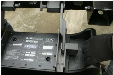
The image shows the connection of the frame to the first Mantas. Please note the use of the S-shaped bar (code V861).
