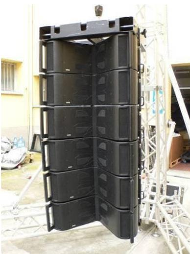
A six-element line-array ready to be lifted up to the working position
