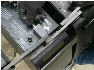
Place the back bar in position and release the pin in order that both this bar and the previous one are locked to the loudspeaker. Repeat this procedure for the other side and for all the loudspeakers on the dolly.
