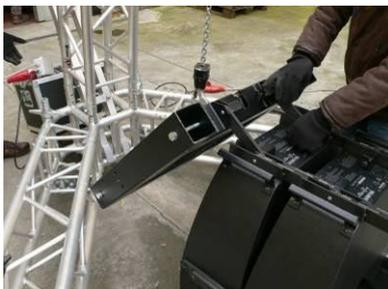
Once all the loudspeakers on the dolly are connected to the rear, lower the frame in order to connect it to the front of the first loudspeaker. Prepare two main frame side connecting bars (V 556).
