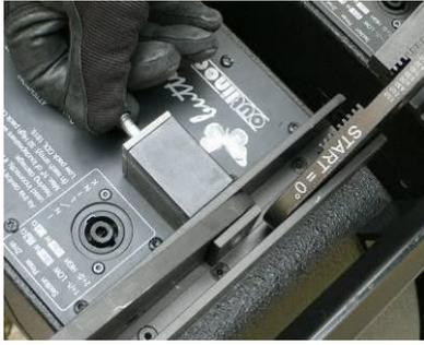
The mechanisms on the loudspeakers allows the user to pull out only half of the pin. In this way it is possible to connect the following loudspeakers without unhooking the previous ones. Bring the graduated back connection bar close to the pin and pull it out only a half.
