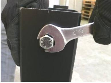
Remove the two M14 screws from the main frame.
