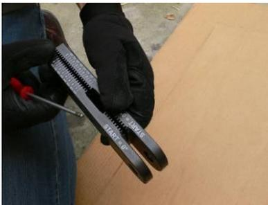
When the screw is sufficiently loose, separate the two parts with the small teeth in order that they can rotate.
