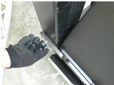
After checking that the cable connected to the frame is not in tension, unscrew the handles of the side connections bars to the frame (V556).
