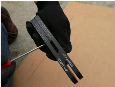
Splay angle selection: partially loosen the screw on the side connection bar using a 4 mm (approx 5/32”) hex key in order to be able to rotate the two parts.
