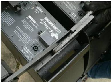
Slightly screw the handle in order to avoid any accidental movement of the pin for safety.
