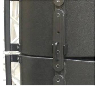
After lifting the first group of loudspeakers, bring the second flight case to the flown system.
