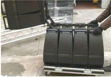
Lower the entire system in order to put the loudspeakers on the dolly.
