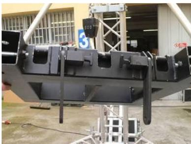
Position the first two back connection bars (V568 for Butterfly, V861 for Mantas): pull the handle to extract the pin, place the bar and release the handle in order to set the pin in its normal working position.
