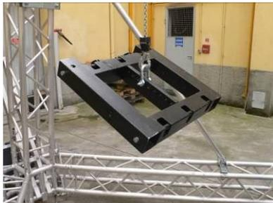
Raise the frame in order to prepare connection of the first group of loudspeakers.
