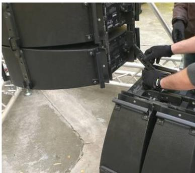
Connect the back bar hooked to the last flown loudspeaker to the first loudspeaker on the dolly. Connect the back of the loudspeakers on the dolly as shown for the first group of loudspeakers.
