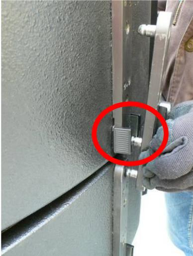
Insert the side connection bar into its location. Slide the safety mechanism upwards, slide inside the connection bar and release the spring mechanism.
