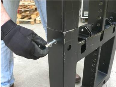
Insert the two M14 screws in their original place in order to firmly connect the two parts together.
