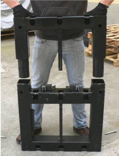
Insert the extension in the main frame as shown in the pictures. The round noses will go into the square tubes.
