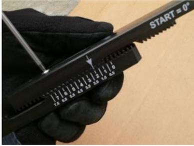
Select the desired splay angle according to the simulation made in OpenArray and fasten the screw using a small torque. The two parts have to be firmly coupled.
