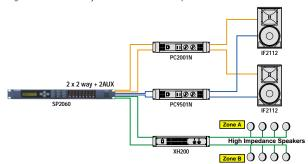
Using the configuration [2x2Way + 2Aux] built into the SP2060 and driving separate power amps for each of the high and low ranges for the main speakers provide pure high-definition sound. Also, two auxiliary lines are supplied to distribute the sound to two separate locations such as a lobby and a dressing room, and can connect the XH200 installation-use power amp to high-impedance speakers. This way, speaker processing for both main and installation use can be performed with one SP2060.
