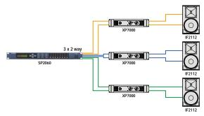
This is an example of a simple connection setting in which the signal is distributed to three speakers. The configuration [3x2-way] installed in the SP2060 is used, and power amps are provided for each speaker. The highs and lows are driven by the two channels of each amp.
